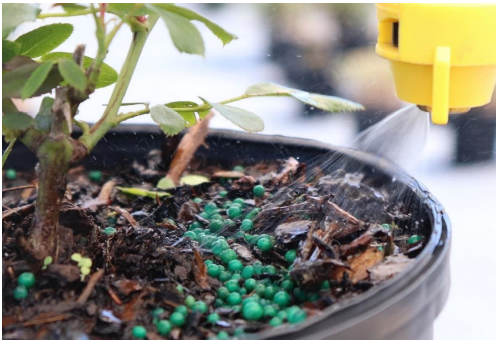
A single off-center flat fan nozzle was positioned 2.5 cm above the substrate and at the edge of the pot. The distal edge of the spray pattern reached the base of the stem in the center of the pot.
